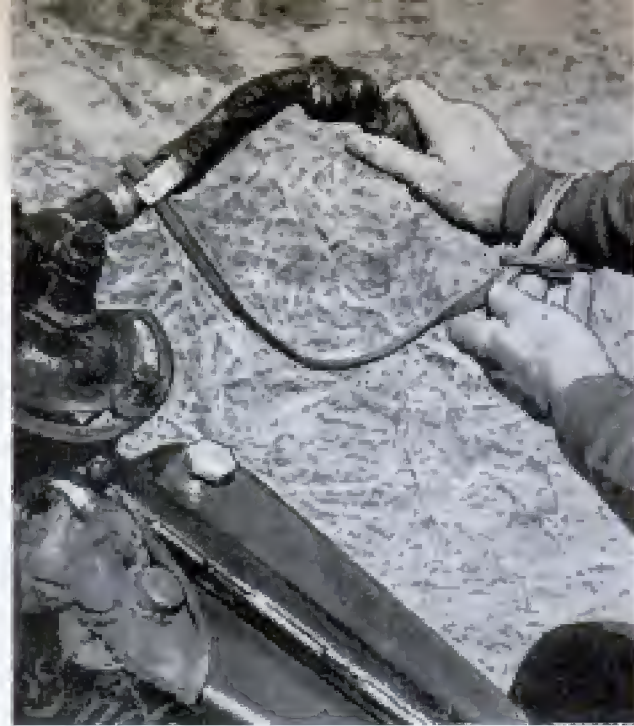
Safety rules require an automatic device to stop the engine if the rider is thrown off. When the thing is pulled from the handle-bar clip, ignition is grounded
